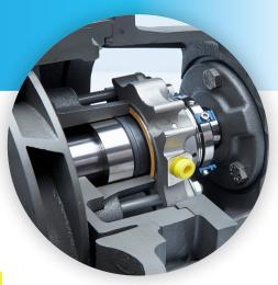
is conducted to the product side and the cooled sealing water flows back from the product side to the atmosphere side, driven by the rotary motion of the shaft. The seal acts like a heat exchanger. The typically obligatory thermosiphon container for dual action mechanical seals is not required.
